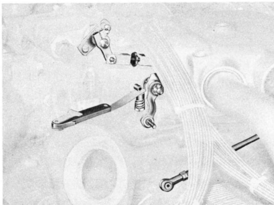
Figure 5-5. Setting Idle Adjusting Screw at Injector Stop Pin
