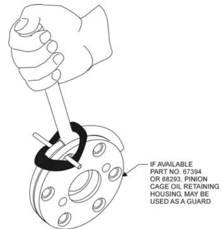
Figure 4. Crankshaft Propeller Flange Showing Installation of Stretch Seal Using a Guard Over the Front of the Flange
