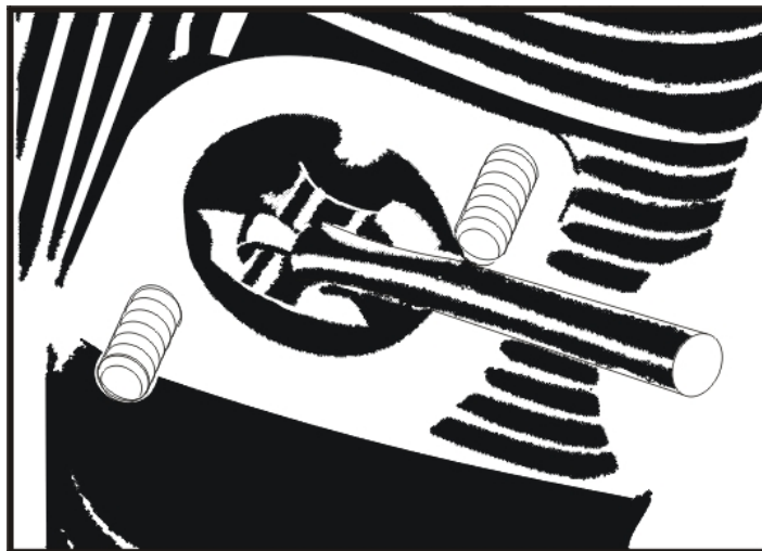
Figure 11. View Through Exhaust Port Showing Mechanical Fingers Holding Valve Stem
