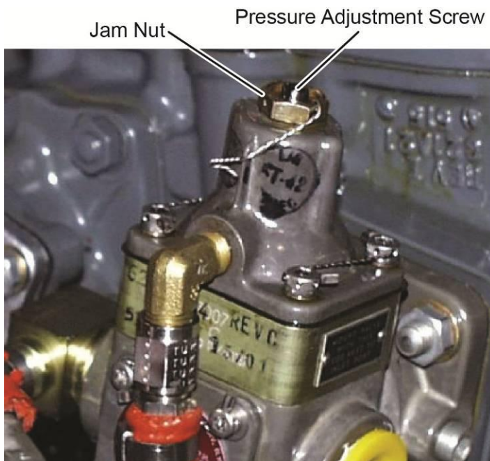
Figure 1 Pressure Adjustment Screw with Jam Nut
