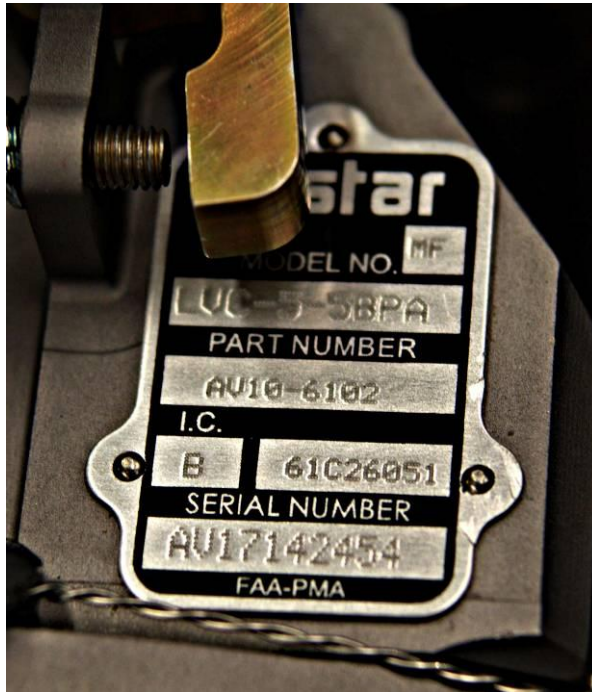
Figure 3 Carburetor Data Tag
