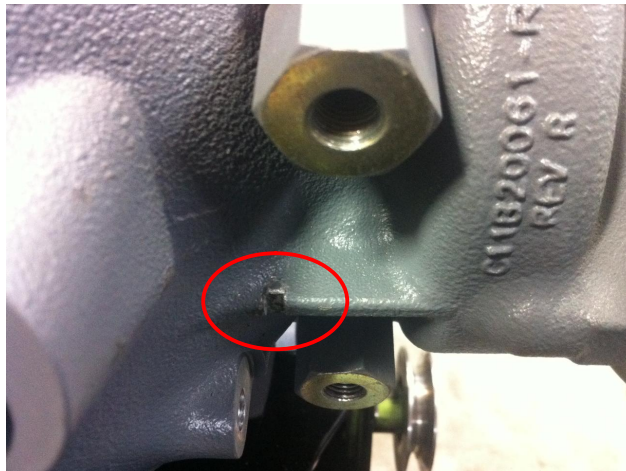
Figure 1 Tight Fit in Nose Clearance - Airframe Bracket
