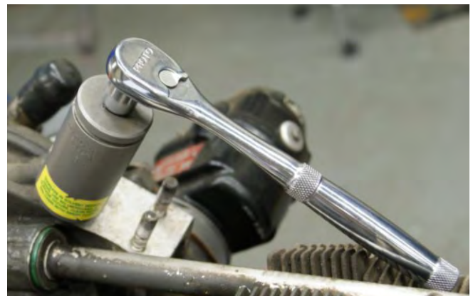
Figure A-2 Stud Remover Tool
