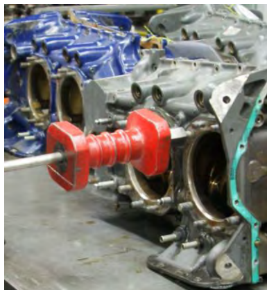
Figure 3 Attach the Slide-Hammer to a Base Stud
