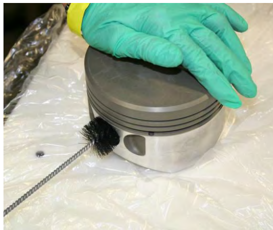
Figure 1 Cleaning the Piston Bore with a Soft Bristle Non-Metallic Brush
