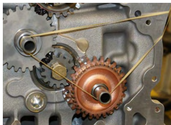
Figure 85 Rubber Band to Hold Crankshaft Idler Gears
