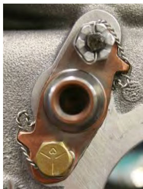
Figure 16 Safety Wire on the Crankshaft Idler Gear Shaft
