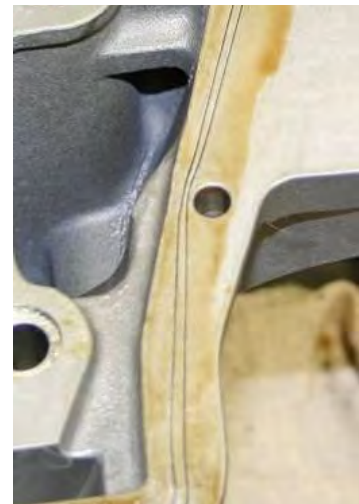
Figure 71 Placement of Silk Threads Along Inside Edge of Crankcase Flange
