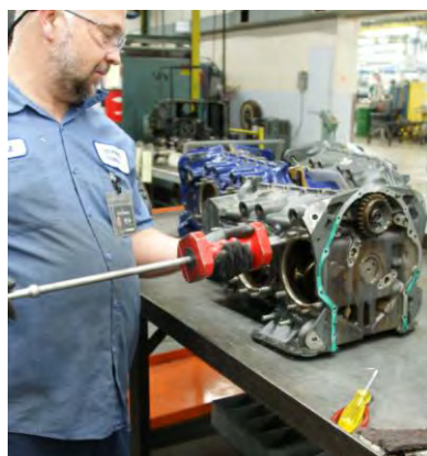
Figure 4 Strike the Slide Part of the Tool Against the Back of the Tool
