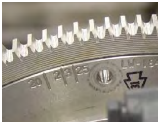
Figure 4 Timing Marks on the Starter Ring Gear Support
