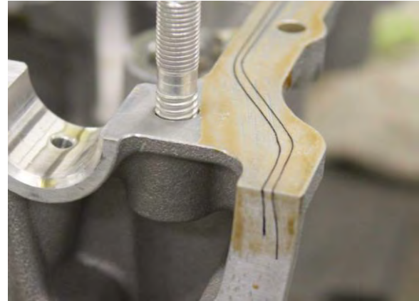
Figure 73 Silk Thread Extending into the Rear End of the Crankcase
