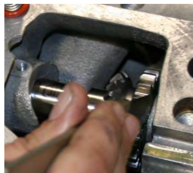
Figure 57 Shim Between Spacer and Crankcase – Backlash Check
