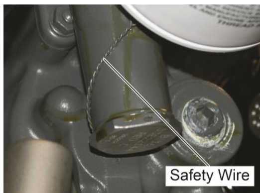
Figure 7 Safety Wire on the Thermostatic Oil Cooler Bypass Valve
