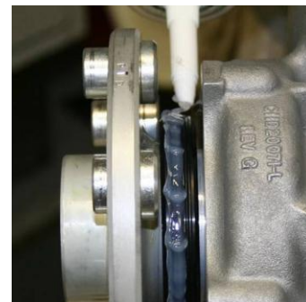
Figure 84 Apply the Sealant to the Oil Seal
