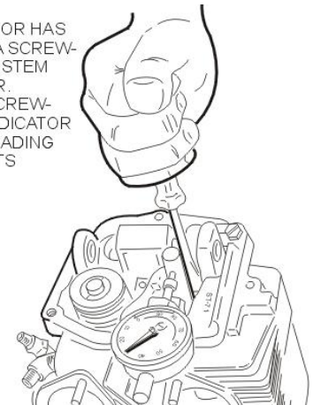
Figure 9 Pushing Valve Stem and Adapter Post Toward Dial Indicator
