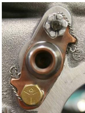
Figure 17 Safety Wire on the Crankshaft Idler Gear Shaft
