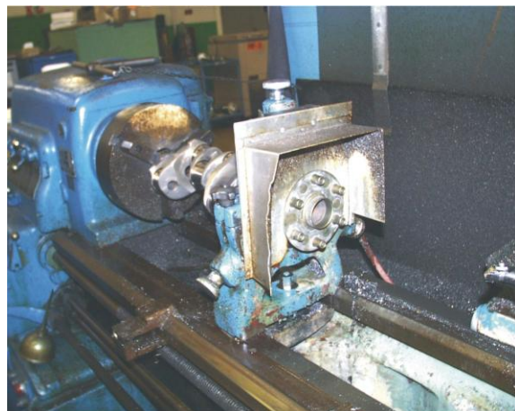
Figure A-8 Crankshaft Clamped in Chuck Jaws
