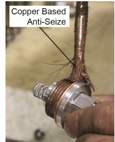
Figure 6 Apply Copper Based Anti-Seize to Threads
