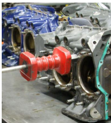
Figure 4 Attach the Slide-Hammer to a Base Stud
