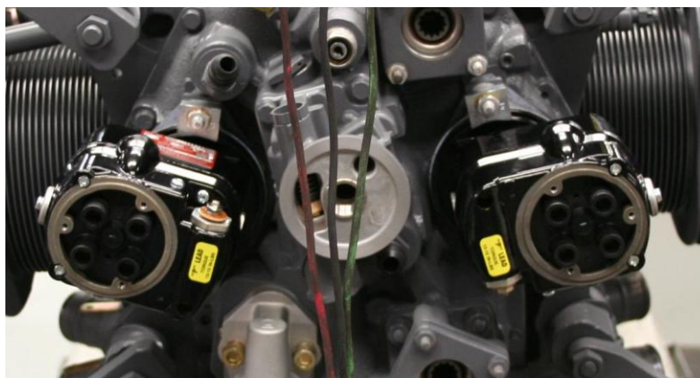
Figure 3 Typical Magneto Position
