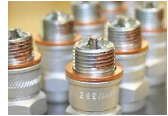
Figure 4 Copper-Based Anti-Seize Applied to Spark Plug Threads
