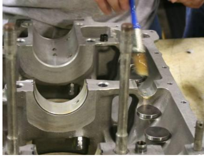
Figure 70 Lubricant Application to Camshaft Bearing Saddle in Crankcase Half
