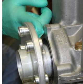
Figure 85 Spread the Excess Sealant
