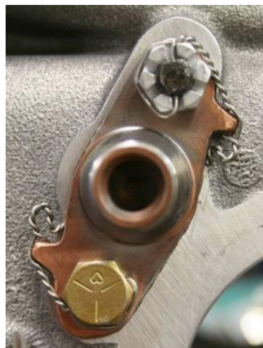
Figure 52 Safety Wiring the Crankshaft Idler Gear Shaft
