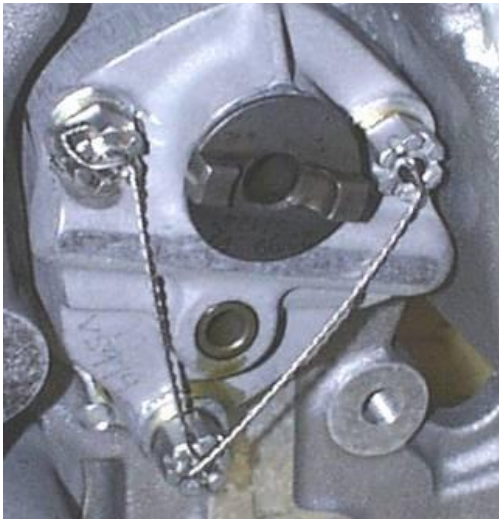
Figure 3 Safety Wire Oil Pump Fasteners
