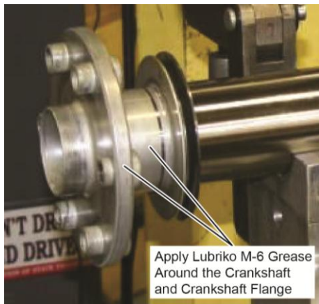
Figure 45 Apply Lubriko M-6 Grease Around the Crankshaft and Crankshaft Flange
