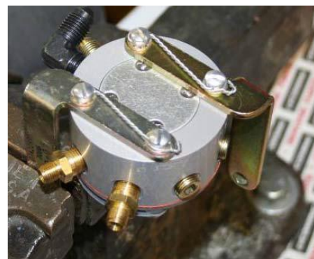
Figure 13 Safety Wire the Screws
