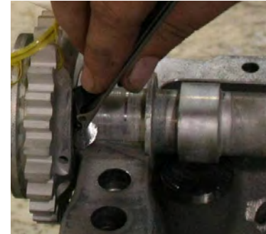
Figure 71 Camshaft End Play Clearance Check
