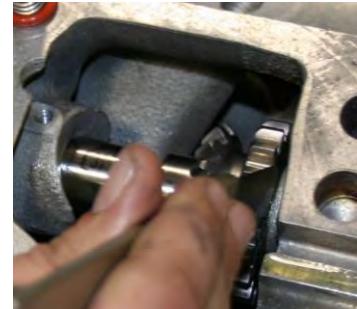
Figure 66 Shim Between Spacer and Crankcase – Backlash Check
