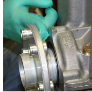
Figure 90 Spread the Excess Sealant
