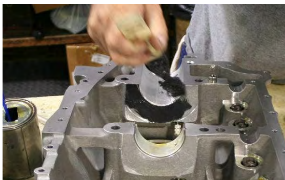
Figure 74 Thrust Bearing Surfaces of Each Crankcase Half
