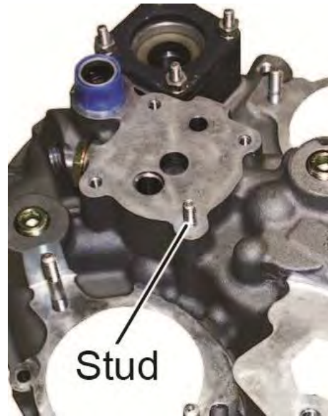
Figure A-7 Stud Driven Height 0.60 to 0.64 in.(15.2 to 16.3 mm).
