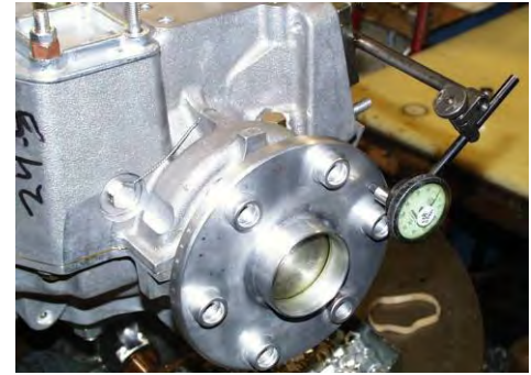
Figure 95 Crankshaft Endplay Check
