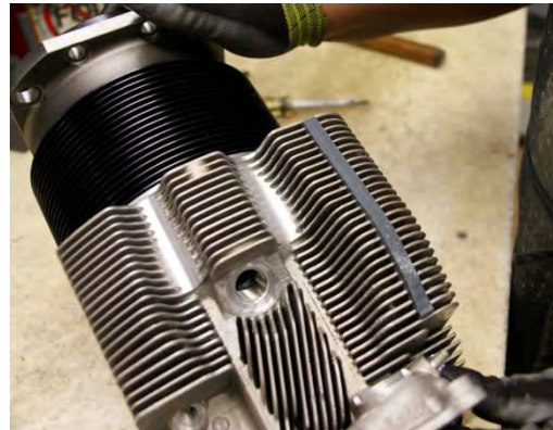
Figure A-5 Fin Stabilizer Installed on Cylinder
