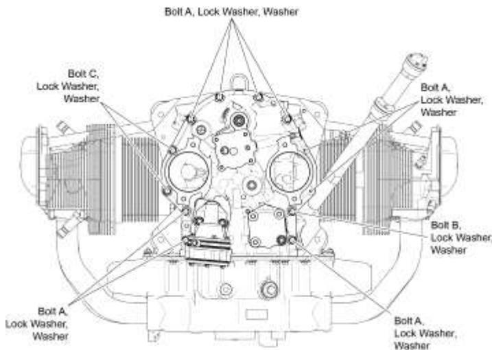
**Figure 1****Hardware on External Side of Accessory Housing**
