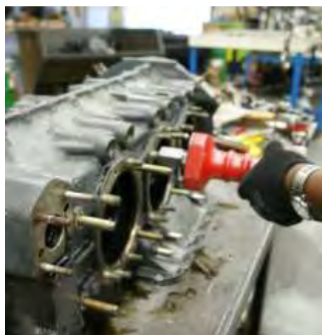
Figure 5 Attach the Slide-Hammer to a Base Stud
