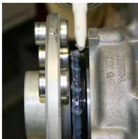
Figure 104 Apply the Sealant to the Oil Seal
