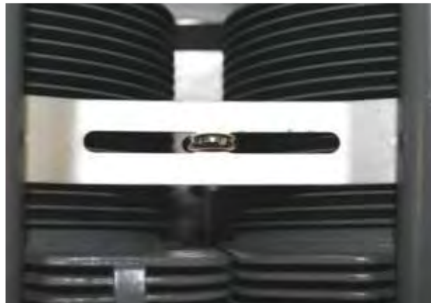
Figure 42 Intercylinder Baffle Installed on Three Fins
