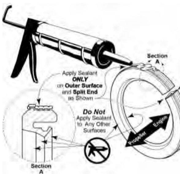
Figure 8 Where to Apply Sealant
