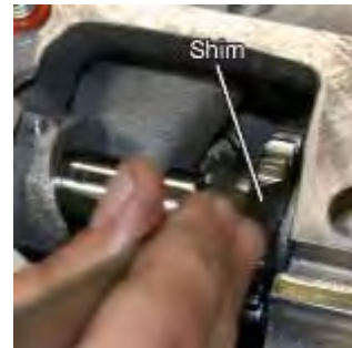
Figure 78 Shim Between Spacer and Crankcase – Backlash Check
