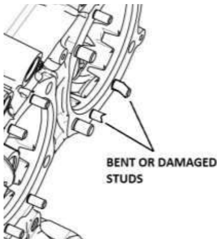
Figure A-1 Damaged Studs
