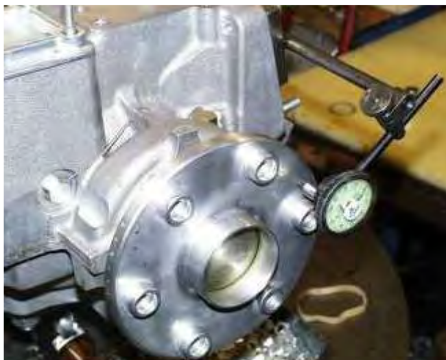
Figure 101 Crankshaft End Play Check
