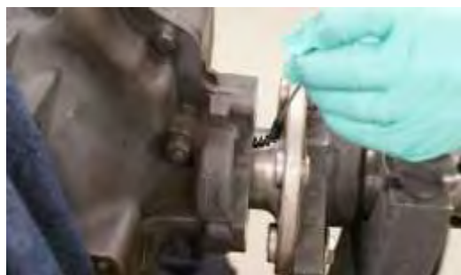
Figure 6 Using Spiral Brush on Hard Deposits
