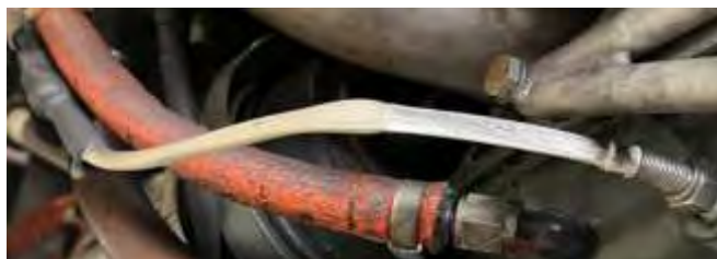
Figure 38 Correct Installation Cable is Smooth and Not Twisted
