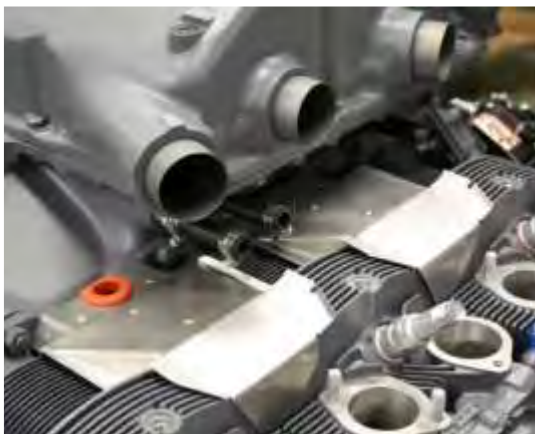
Figure 41 Placement of Intercylinder Baffle on Down Exhaust Engines
