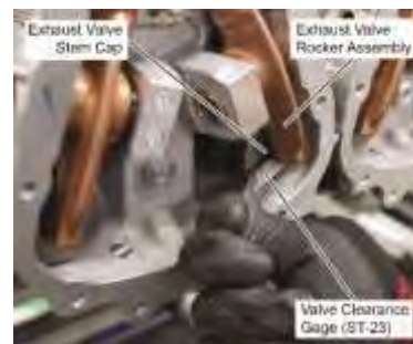
Figure 38 Measuring Dry Tappet Clearance
