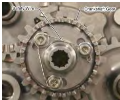
Figure 118 Safety Wire the Crankshaft Trigger Gear Assembly Screws
