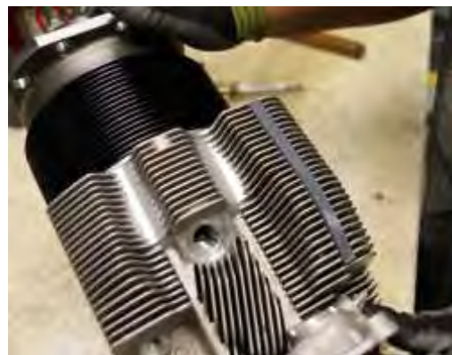
Figure A-5 Fin Stabilizer Installed on Cylinder
