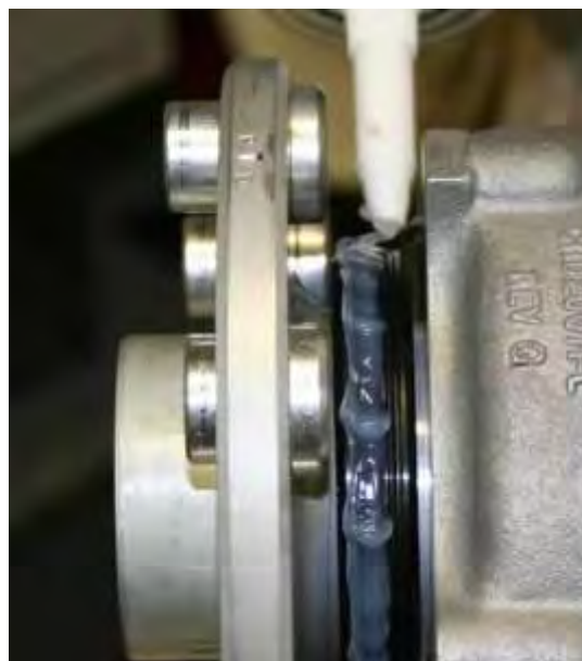
Figure 9 Applying Permatex® Optimum Max Flex Black (P/N 27037)
