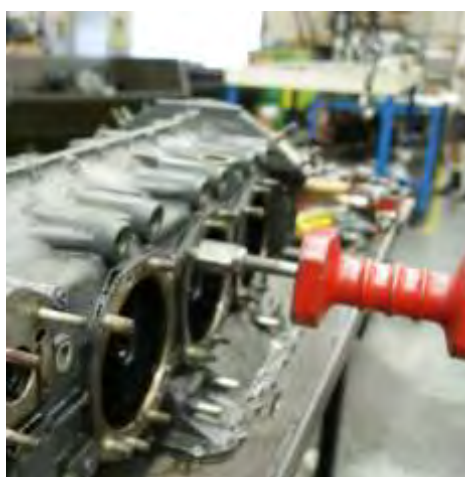
Figure 6 Strike the Slide Part of the Tool Against the Back of the Tool
