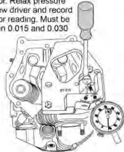
Figure 9 Pushing Valve Stem and Adapter Post Toward Dial Indicator
