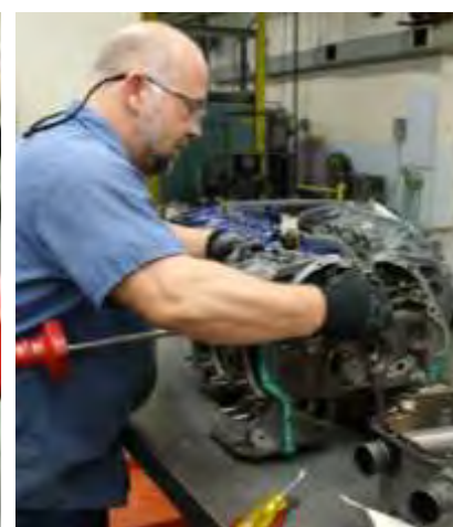
Figure 7 Separate the Crankcase Halves
