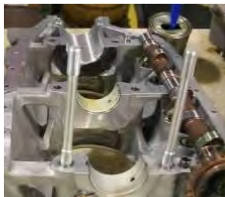
Figure 85 Thrust Bearing Surfaces and Main Bearings of Each Crankcase Half
