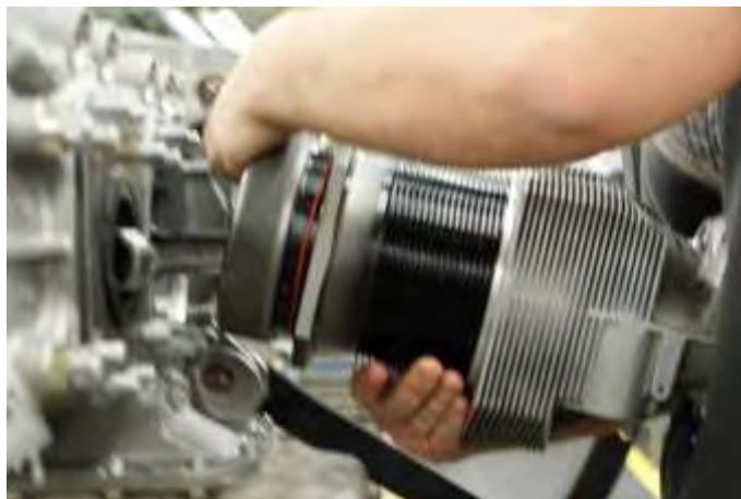
Figure 29 Install the Cylinder
