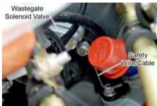
Figure 9 Safety Wire/Cable on Wastegate Solenoid Valve Bolt
