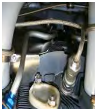
Figure 44 Loose Fit of Intercylinder Baffle
