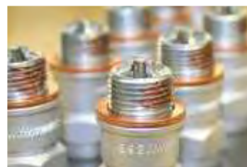
Figure 6 Copper-Based Anti-Seize Applied to Spark Plug Threads
