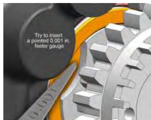
Figure 115 Crankshaft Trigger Gear Assembly Pilot Flange
