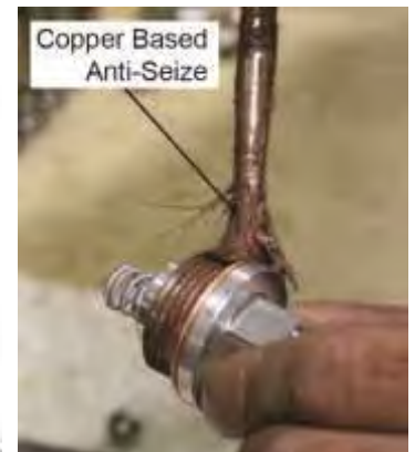
Figure 6 Apply Copper Based Anti-Seize to Threads
