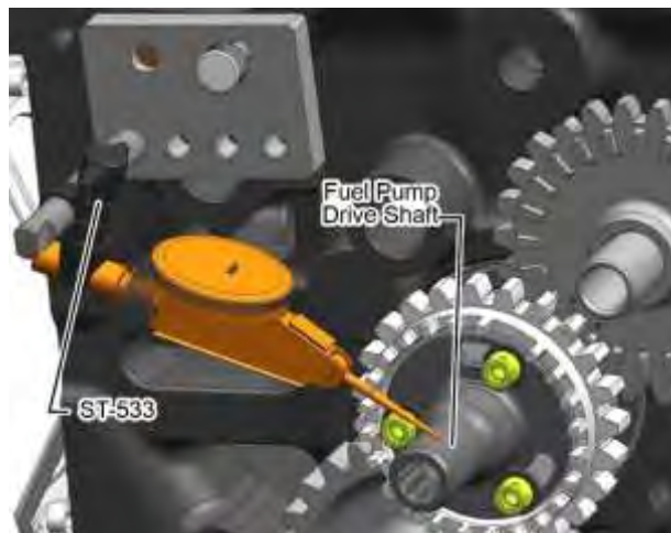
Figure 117 Fuel Pump Shaft Drive Indicator Mount (ST-533)
