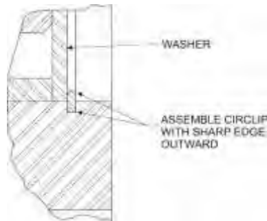
Figure 64 Assembly of Circlips in Counterweight
