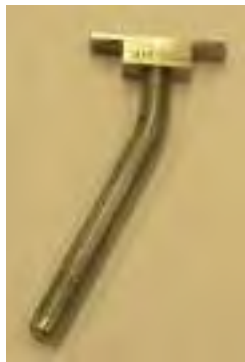
Figure 66 Circlip Check Gage P/N 64892-2
