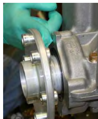
Figure 28 Spread Sealant in Gap Between Case & Seal
