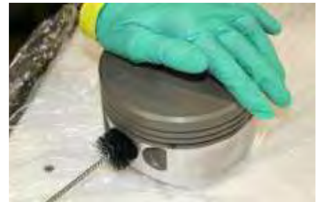
Figure 2 Cleaning the Piston Pin Bore with a Soft Bristle Non-Metallic Brush
