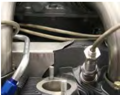
Figure 43 Correct Tight Fit of Intercylinder Baffle
