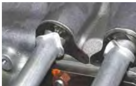
Figure 35 Correctly Aligned Shroud Tube Springs
