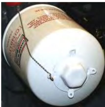
Figure 5 Safety Wire on Oil Filter
