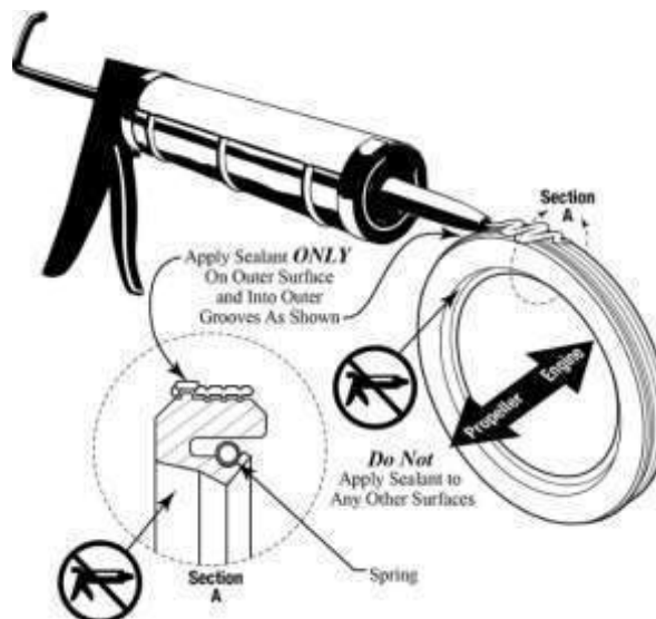
Figure 29 Where to Apply Sealant
