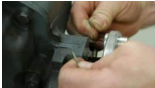
Figure 21 Installing the Spring Behind the Solid-Ring Crankshaft Oil Seal
