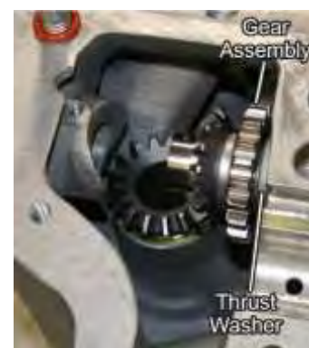
Figure 76 Propeller Governor Idler Gear Assembly and Thrust Washer
