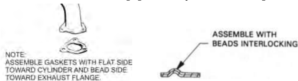
Figure 7 Exhaust Flange Gasket
