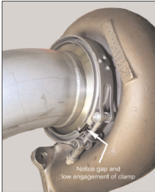
Figure 2 - "V" band Clamp Showing Gap
