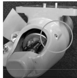
- Picture 2 - Unaffected Mount Castings Have 1) More Generous Radii Geometry Around Nose Opening Cutout and 2) Significantly More Edge Distance Between Timing Mark and Nose Opening Cutout
