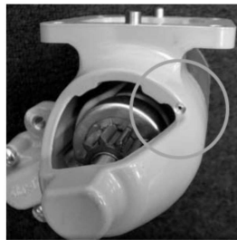
- Picture 1 - Mount Castings on Affected Starters Have 1) Sharper Radii Geometry Around Nose Opening Cutout and 2) Little/No Edge Distance Between Timing Mark and Nose Opening Cutout
