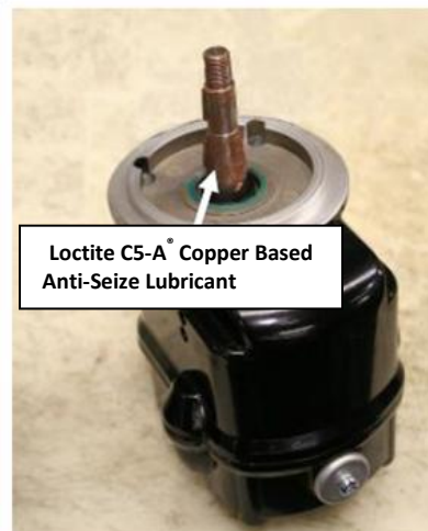
Figure 2 Apply Loctite C5-A ® Copper Based Anti-Seize Lubricant to the Shaft
