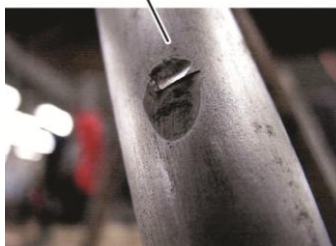
Figure 1 Chafing on Support Rod
