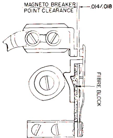
Figure 2 - Adjusting Breaker Point Clearance on Heavyweight Magnetos
