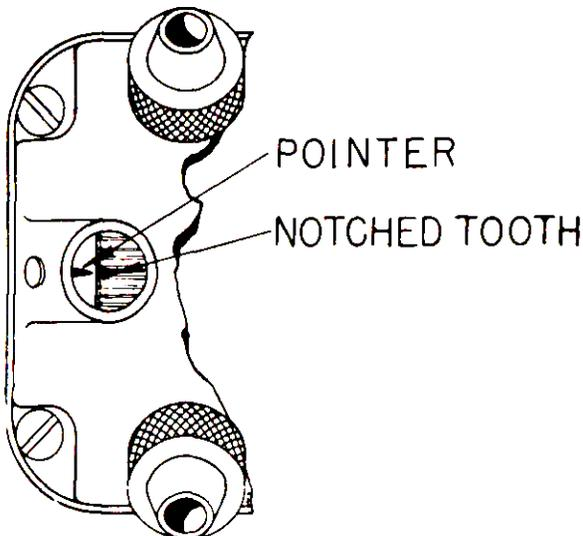
Figure 1 - Alignment of Notched Tooth and Pointer
