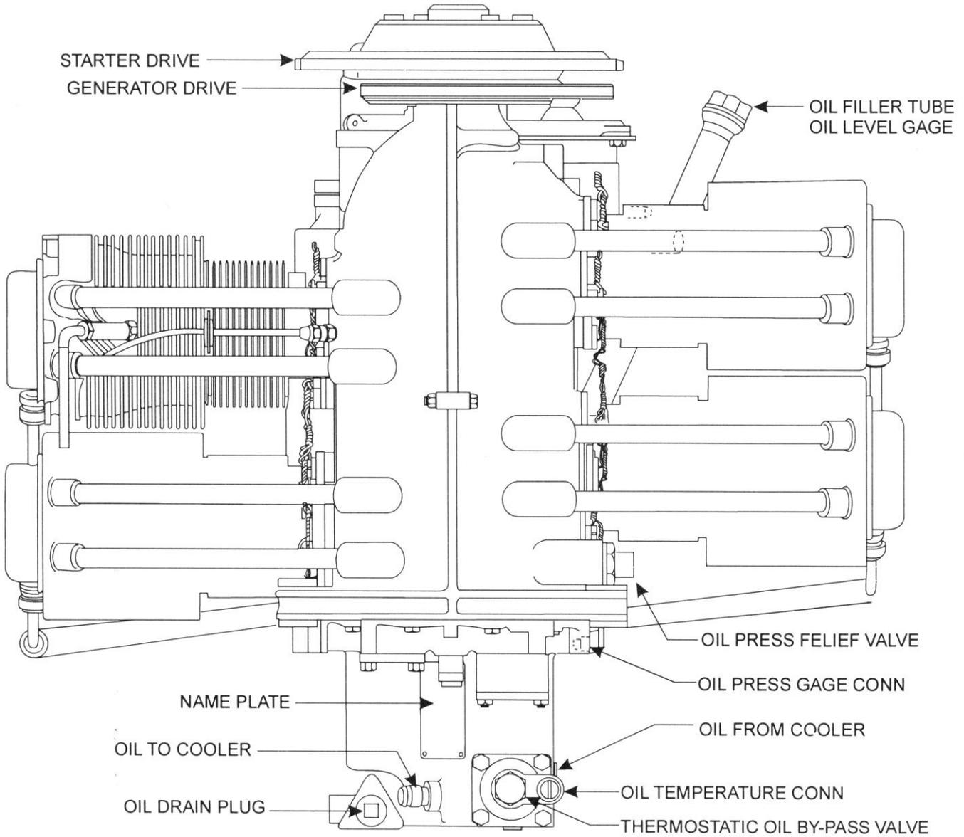
Figure 7-2. Installation Drawing – Forward View – VO-360
