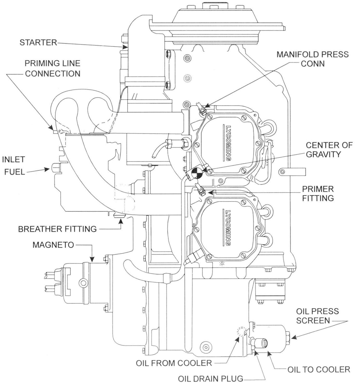
Figure 7-1. Installation Drawing – Right Side View – VO-360
