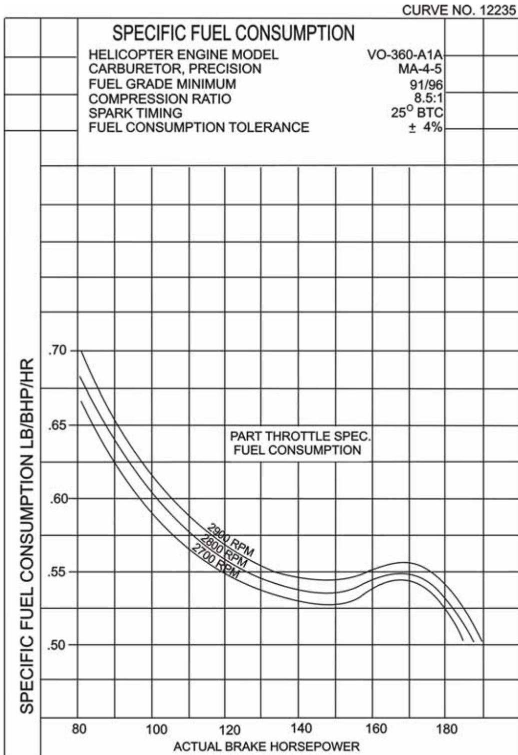
Figure 3-1. Fuel Consumption Curve – VO-360-A1A
