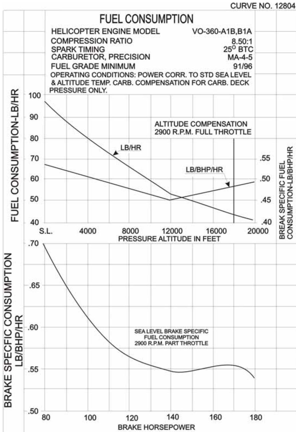
Figure 3-3. Fuel Consumption Curve – VO-360-A1B, -B1A
