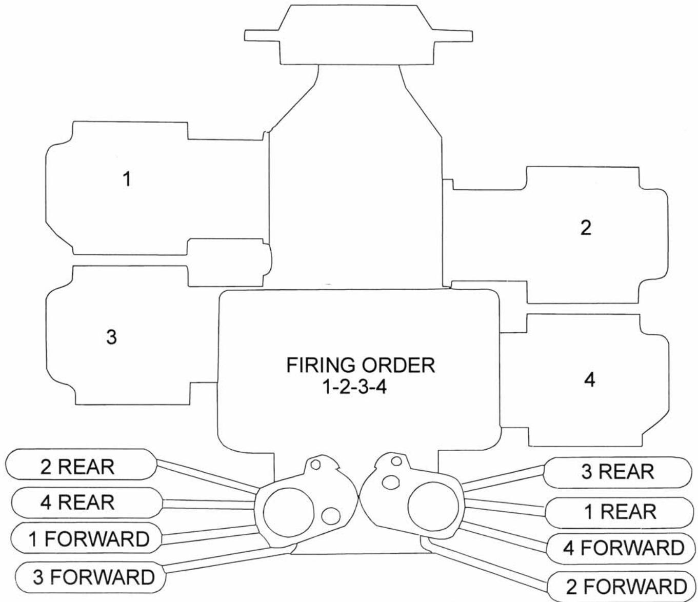
Figure 5-1. Ignition Wiring Diagram
