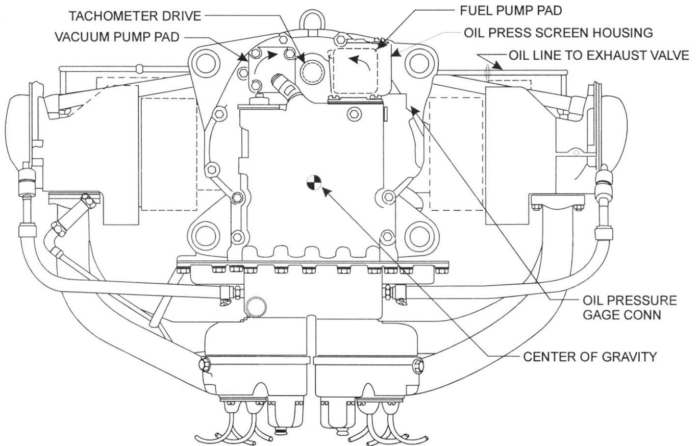
Figure 7-3. Installation Drawing – Bottom View – VO-360
