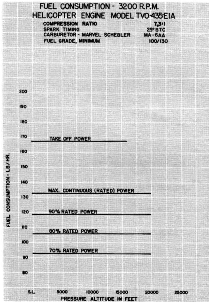
Figure 3-15. Fuel Consumption Curve - TVO-435-E Series
