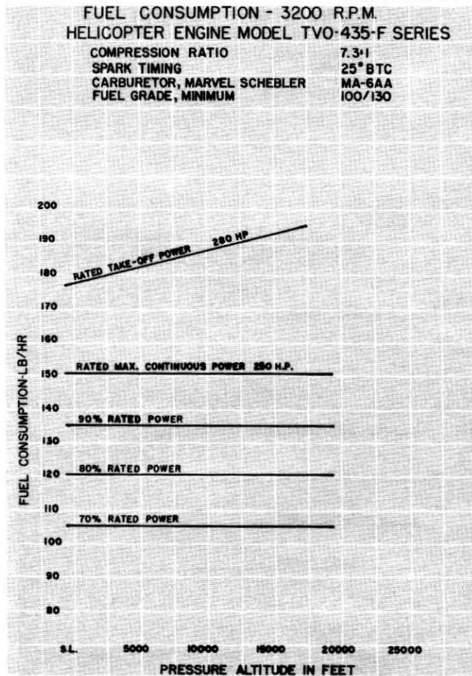
Figure 3-16. Fuel Consumption Curve - TVO-435-F Series
