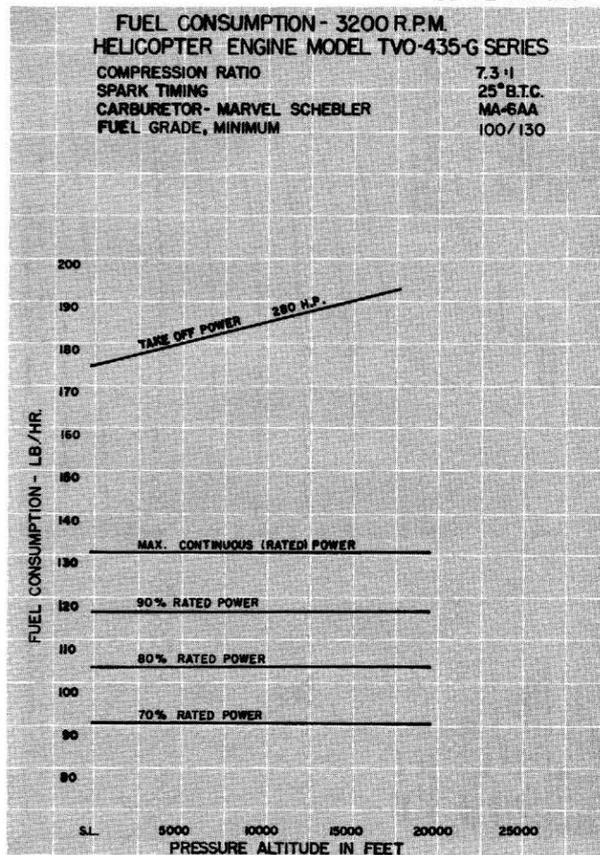
Figure 3-17. Fuel Consumption Curve - TVO-435-G Series
