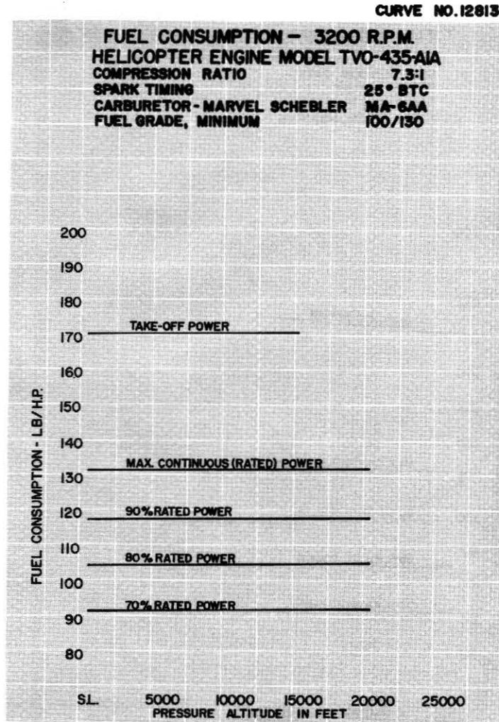
Figure 3-3. Fuel Consumption Curve - TVO-435-A Series
