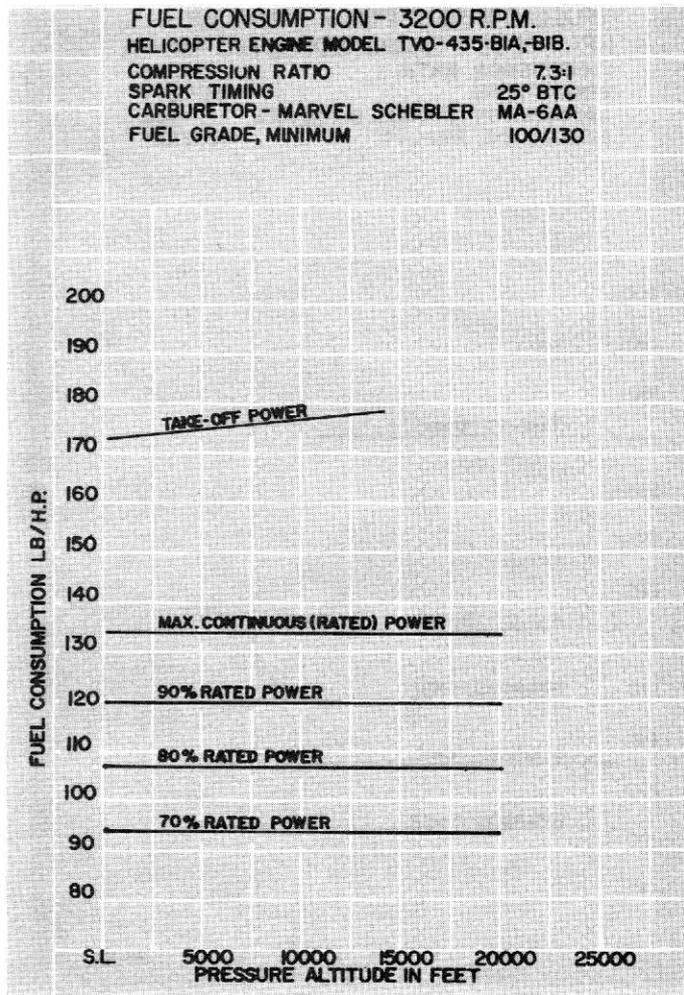
Figure 3-4. Fuel Consumption Curve - TVO-435-B Series
