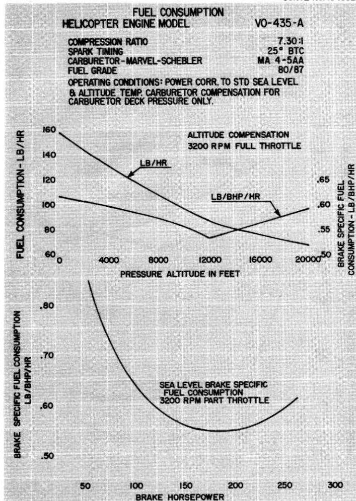
Figure 3-1. Fuel Consumption Curve - VO-435-A Series
