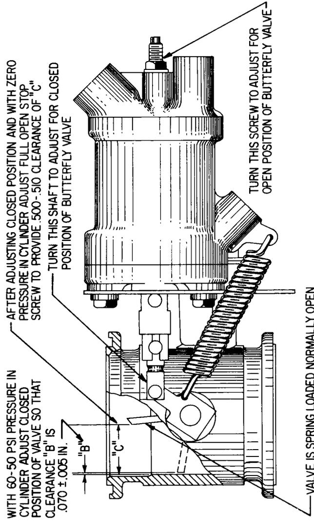
Figure 5-4. Waste Gate Setting - TVO-435-D1A, -D1B, -F1A, -G1A, -G1B
