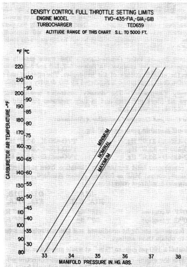
Figure 5-8. Density Control Full Throttle Setting Limits
