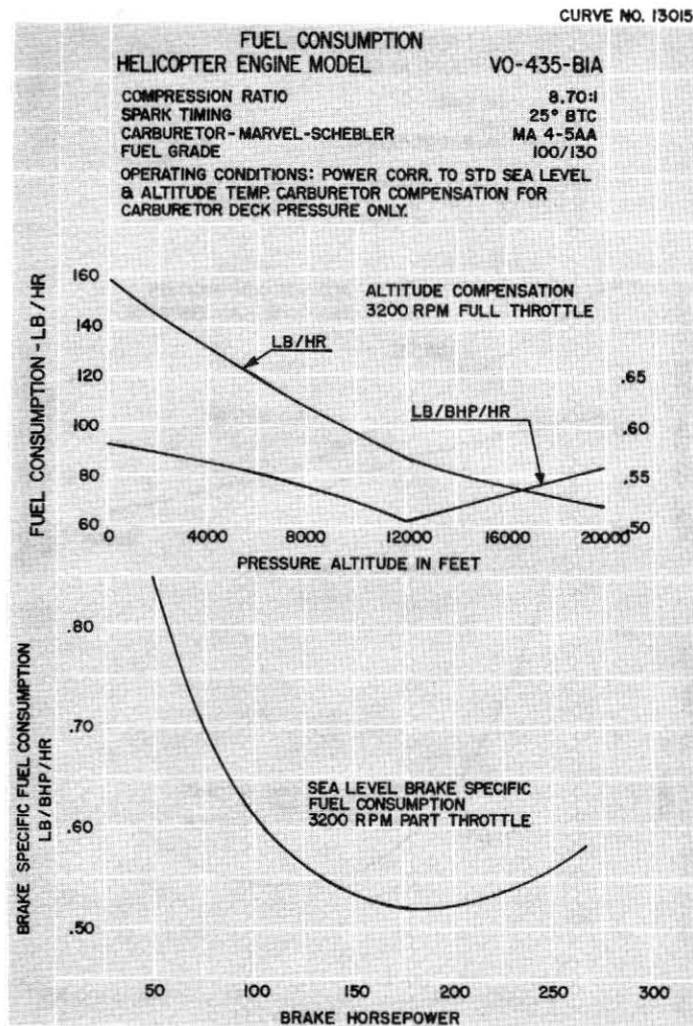
Figure 3-2. Fuel Consumption Curve - VO-435-B Series
