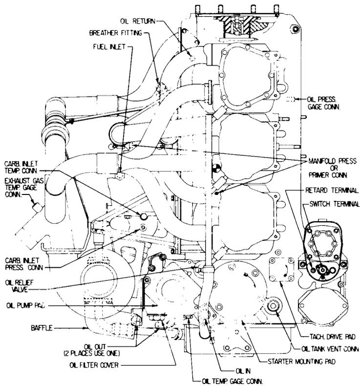
Figure 7-6. Installation Drawing - Right Side - TVO-435-D Series
