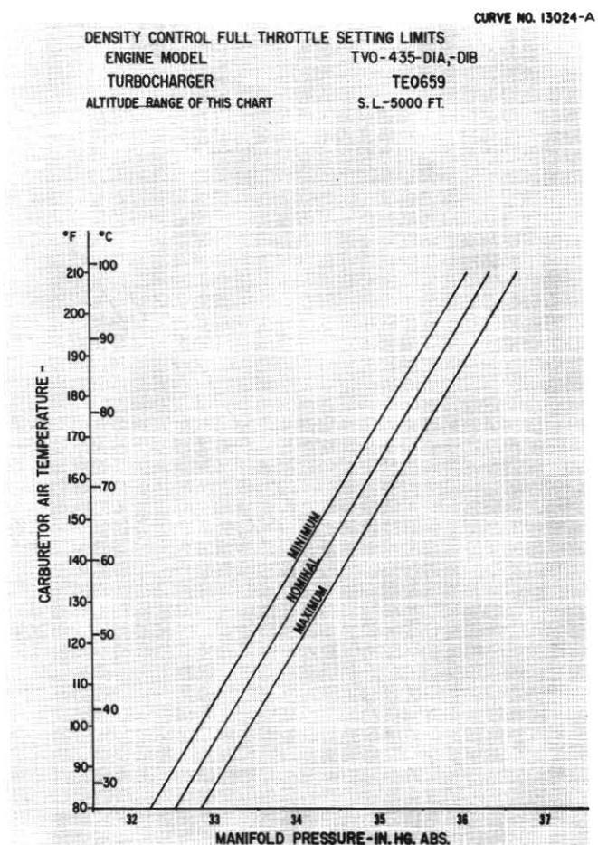
Figure 5-7. Density Control Full Throttle Setting Limits
