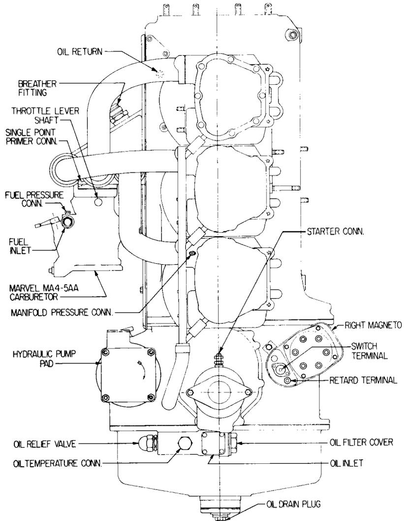
Figure 7-3. Installation Drawing - Right Side - VO-435-B Series
