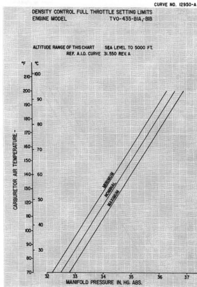
Figure 5-6. Density Control Full Throttle Setting Limits
