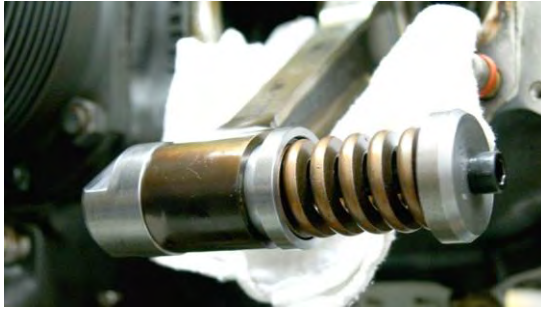
Figure 14 ST-531 Installed in the Connecting Rod
