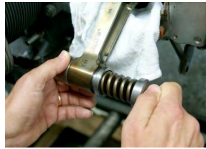
Figure 15 Turn the Bolt Head of the ST-531
