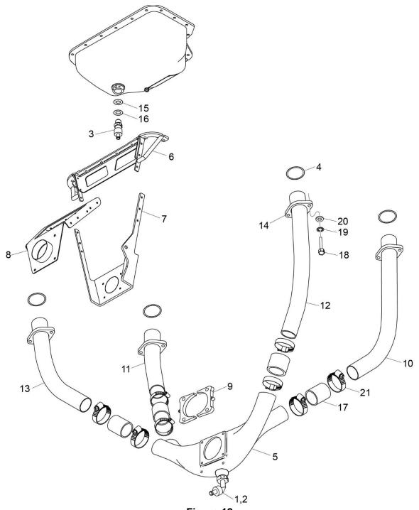
Figure 12 Intake Pipes and Attaching Parts
