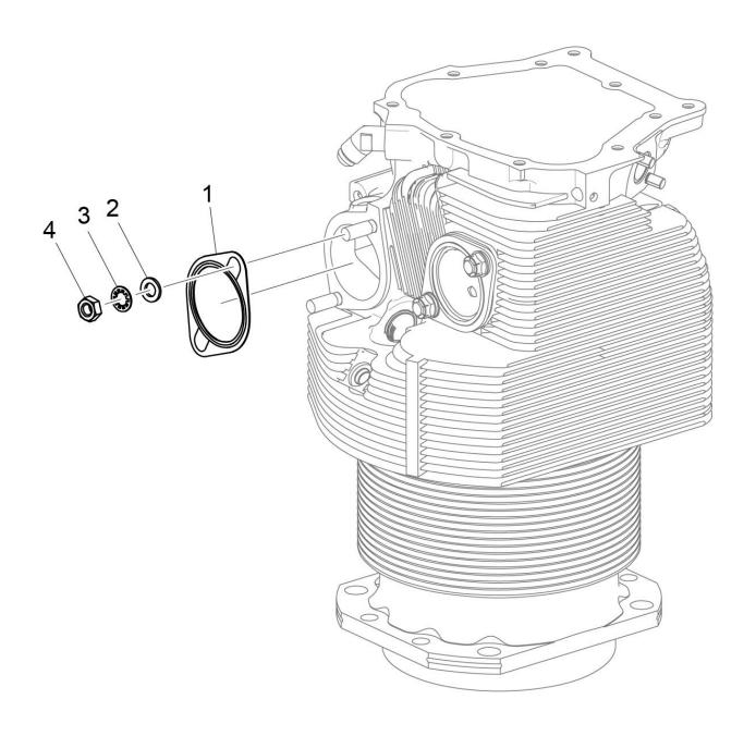
Figure 20 Exhaust Gasket and Flange Attaching Parts
