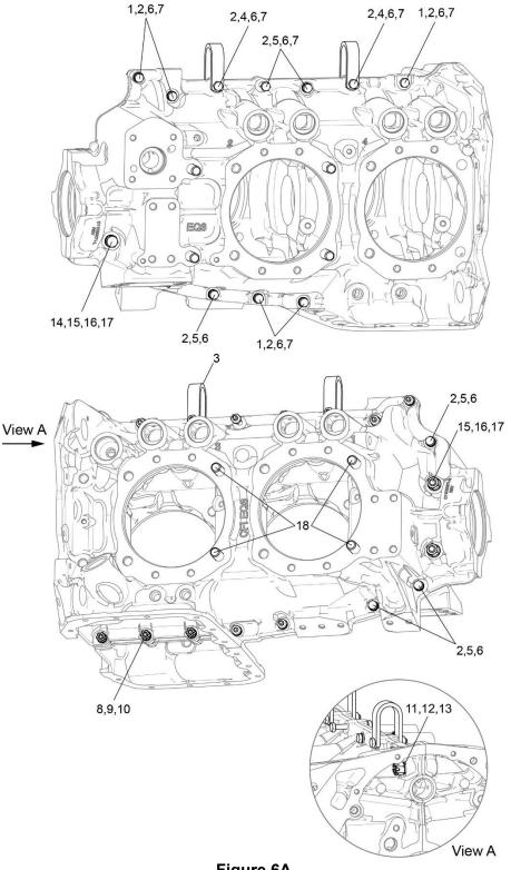
Figure 6A Crankcase Attaching Parts
