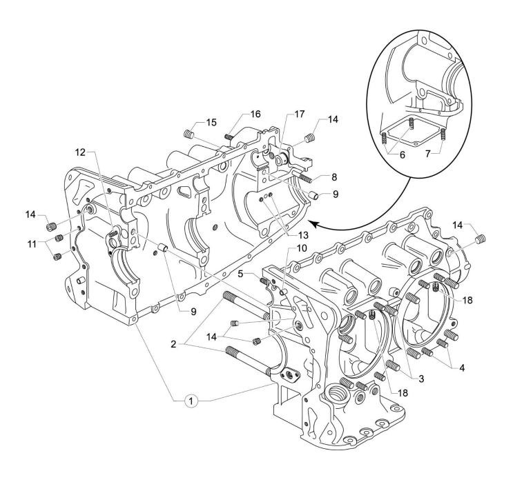
Figure 2 Crankcase Assembly
