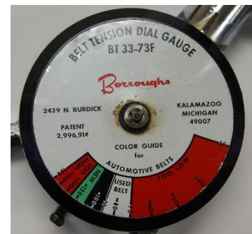
Figure 2 Belt Tension Gage Dial
