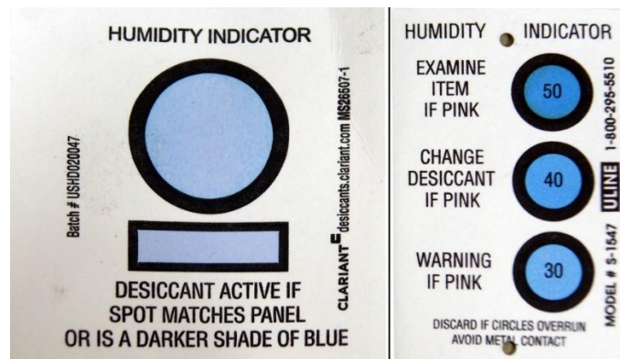
Figure 4 Humidity Indicator Showing No Moisture Present in the Bag
