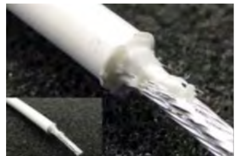
Figure 80 Examples of Burned and Melted Insulation
