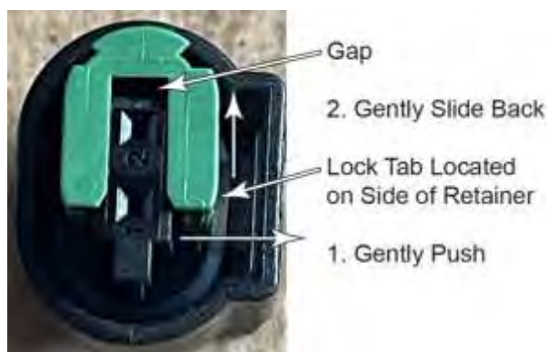
Figure 117 Slide the Second Contact Retainer
