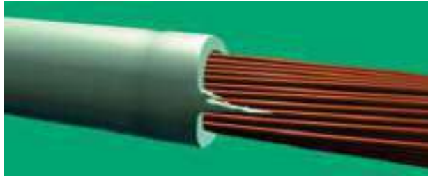
Figure 59 Example of Unacceptable Insulation Jacket
