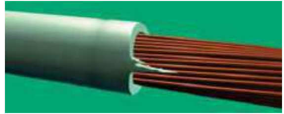
Figure 77 Example of Unacceptable Insulation Jacket
