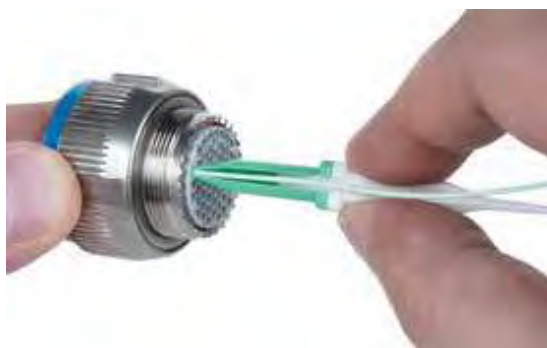
Figure 23 Push the Contact Straight into the Grommet Cavity
