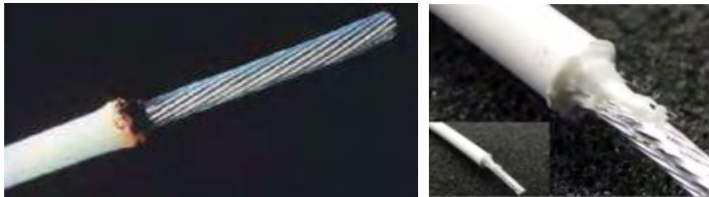
Figure 175 Examples of Burned and Melted Insulation
