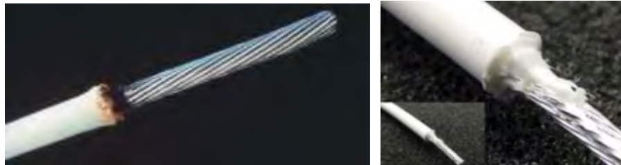
Figure 44 Examples of Burned and Melted Insulation
