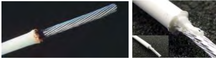
Figure 16 Examples of Burned and Melted Insulation
