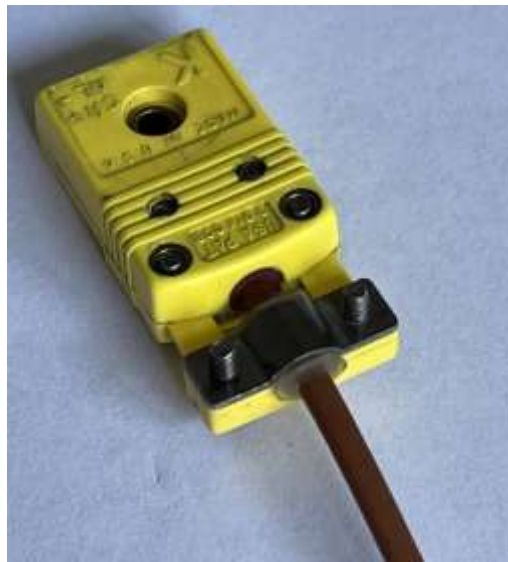
Figure 148 Clamp Back Plate Installation
