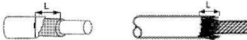
Figure 42 Inter-Tape or Frayed Insulation Exposure
