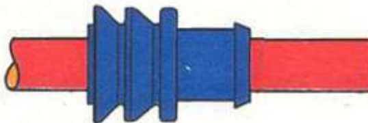
Figure 97 Fit Wire Seals on Wires
