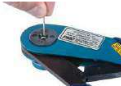
Figure 19 Insert Contact with Wire into Crimping Tool
