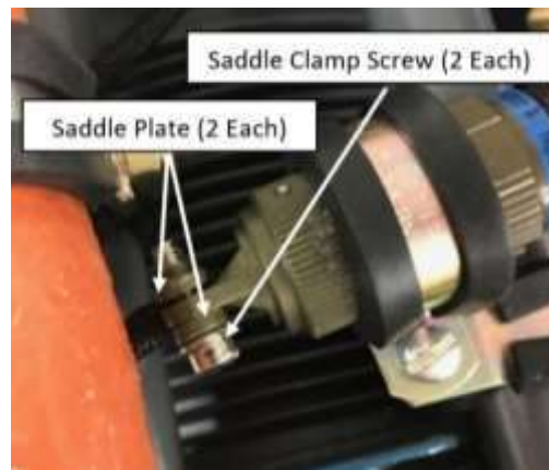
Figure 24 Saddle Clamp Screws and Saddle Plates
