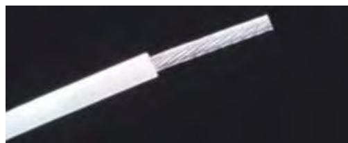
Figure 58 Properly Cut Insulation Jacket
