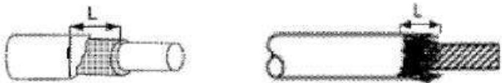
Figure 78 Inter-Tape or Frayed Insulation Exposure
