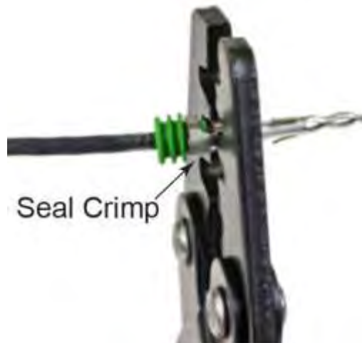
Figure 47 Insert Wire into Terminal
