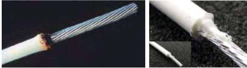
Figure 215 Examples of Burned and Melted Insulation
