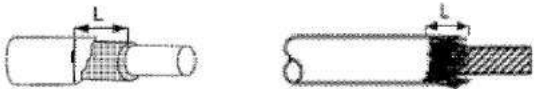
Figure 60 Inter-Tape or Frayed Insulation Exposure
