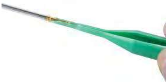
Figure 22 Seat the Retention Shoulder Against the Tip of the Tool
