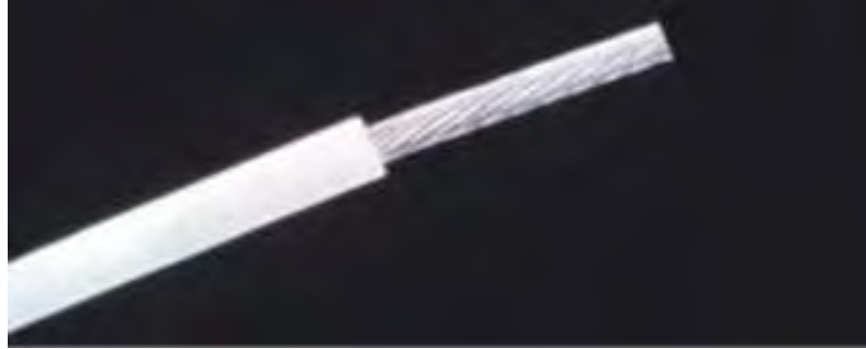
Figure 12 Properly Cut Insulation Jacket
