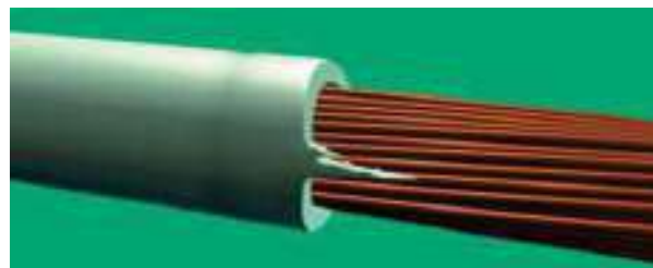
Figure 172 Example of Unacceptable Insulation Jacket
