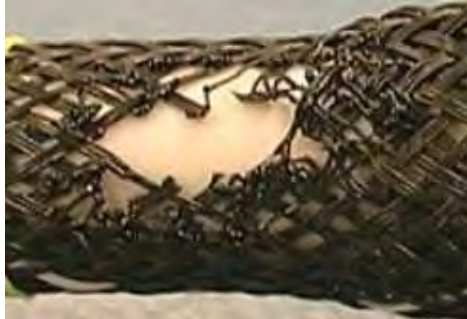
Figure 8 Melted or Heat Damaged Braid
