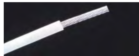
Figure 40 Properly Cut Insulation Jacket
