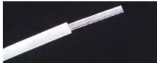
Figure 184 Inspect for Proper Cut
