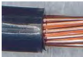
Figure 151 Examples of Unacceptable Wire Strands
