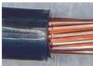
Figure 170 Examples of Unacceptable Wire Strands
