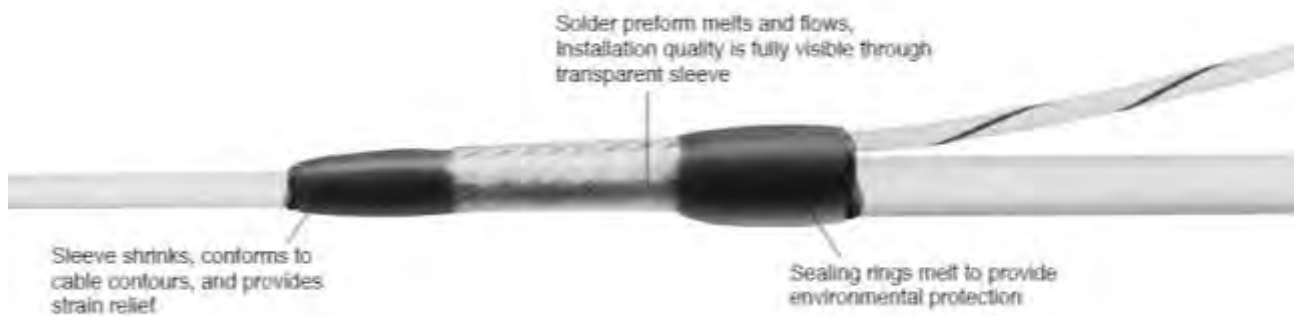
Figure 208 Inspect the Cable Shield Heat Sleeve
