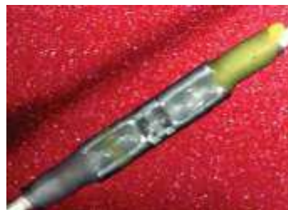
Figure 181 Properly Centered and Shrunk Sealing Sleeve
