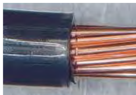
Figure 57 Examples of Unacceptable Wire Strands
