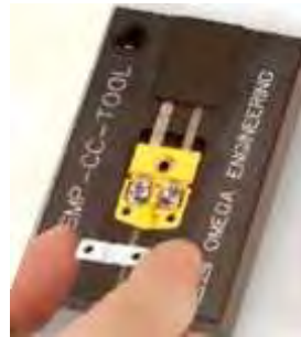
Figure 144 Connector Seating in Assembly Tool
