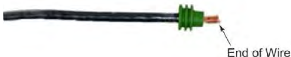
Figure 45 Slide Wire Seal to Flush with Insulation
