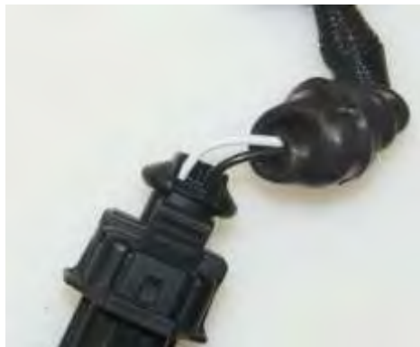
Figure 69 Protective Boot Away from Connector
