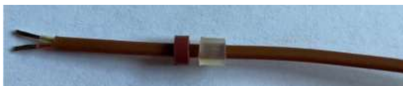
Figure 142 Red and Clear Grommet Installation
