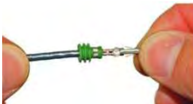
Figure 48 Ensure Terminal and Seal are Secure
