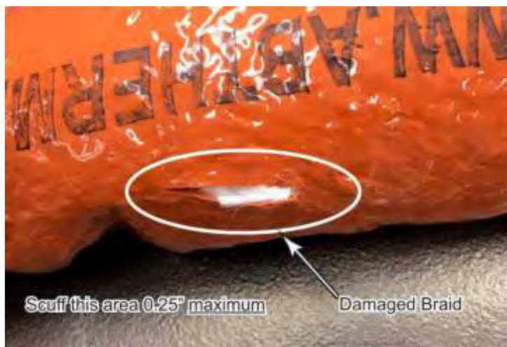
Figure 221 Damage Braiding and Sleeve Preparation
