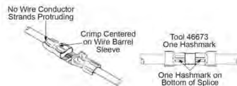
Figure 218 Properly Crimped Terminal and Splice
