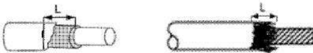
Figure 14 Inter-Tape or Frayed Insulation Exposure
