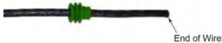
Figure 37 Insert Cable Seal Over Wire
