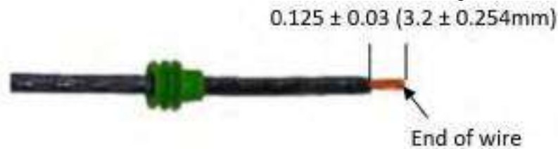
Figure 38 Strip Insulation
