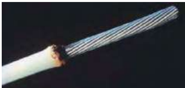
Figure 80 Examples of Burned and Melted Insulation
