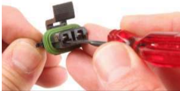
Figure 36 Press the Tang of the Terminal
