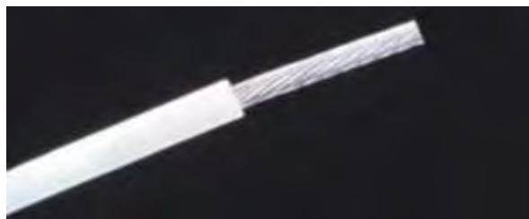
Figure 171 Properly Cut Insulation Jacket
