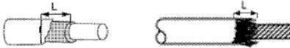
Figure 173 Inter-Tape or Frayed Insulation Exposure
