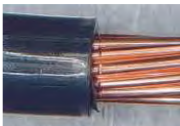
Figure 99 Examples of Unacceptable Wire Strands
