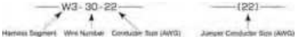
Figure 162 Single Conductor, Unshielded Wire (M22759/43-X-9)
