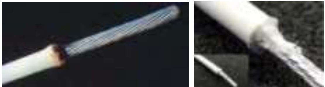
Figure 62 Examples of Burned and Melted Insulation
