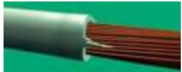
Figure 172 Example of Unacceptable Insulation Jacket
