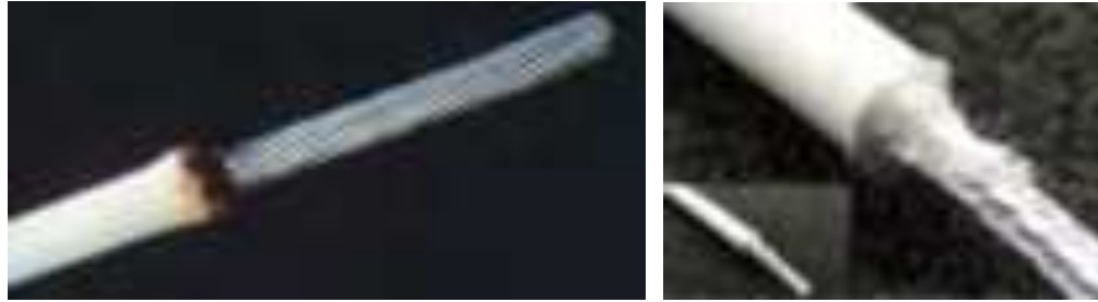
Figure 215 Examples of Burned and Melted Insulation
