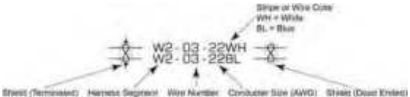
Figure 164 Shielded Twisted Pair Conductor (M27500-XXSP2S23)
