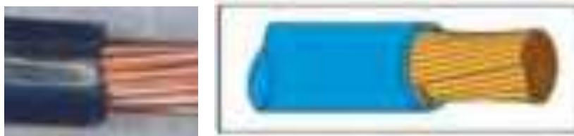
Figure 57 Examples of Unacceptable Wire Strands
