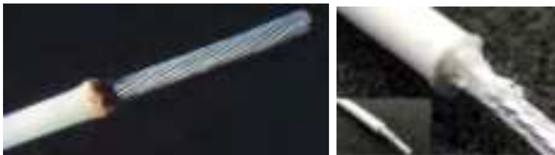
Figure 236 Examples of Burned and Melted Insulation
