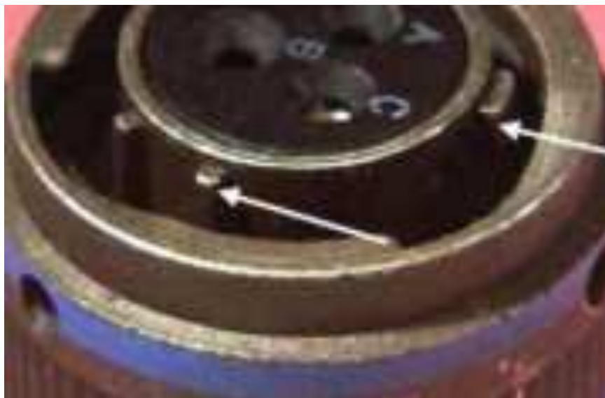
Figure 1 Normal Wear of Keys and Keyways
