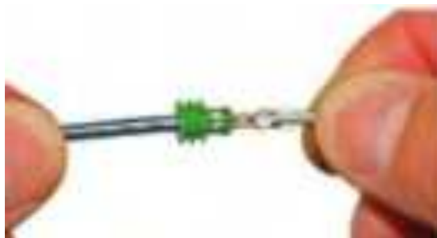
Figure 48 Ensure Terminal and Seal are Secure
