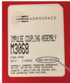
MANUFACTURED DATE LOCATED ON IMPULSE COUPLING REPLACEMENT KIT
