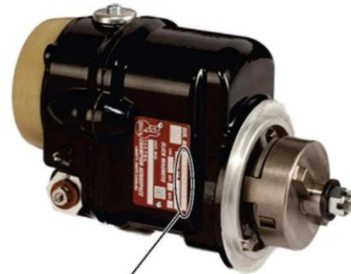
SERIAL NUMBER LOCATED ON MAGNETO DATAPLATE
