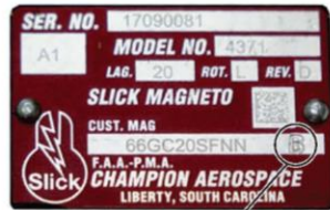
LETTER "B" INDICATES REPAIRED MAGNETO
