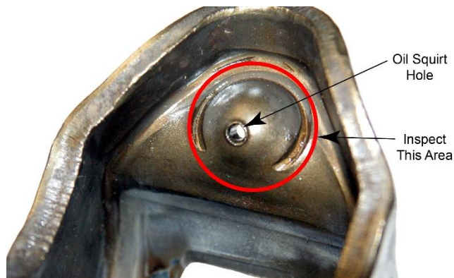
Figure 8 Area to Inspect (Outside of the Rocker Arm)
